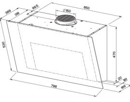
To be installed at a minimum distance from the hob of 45 cm.
