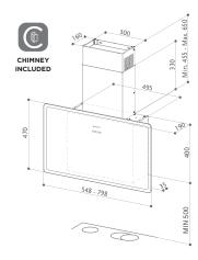
To be installed at a minimum distance from the hob of 50 cm.
