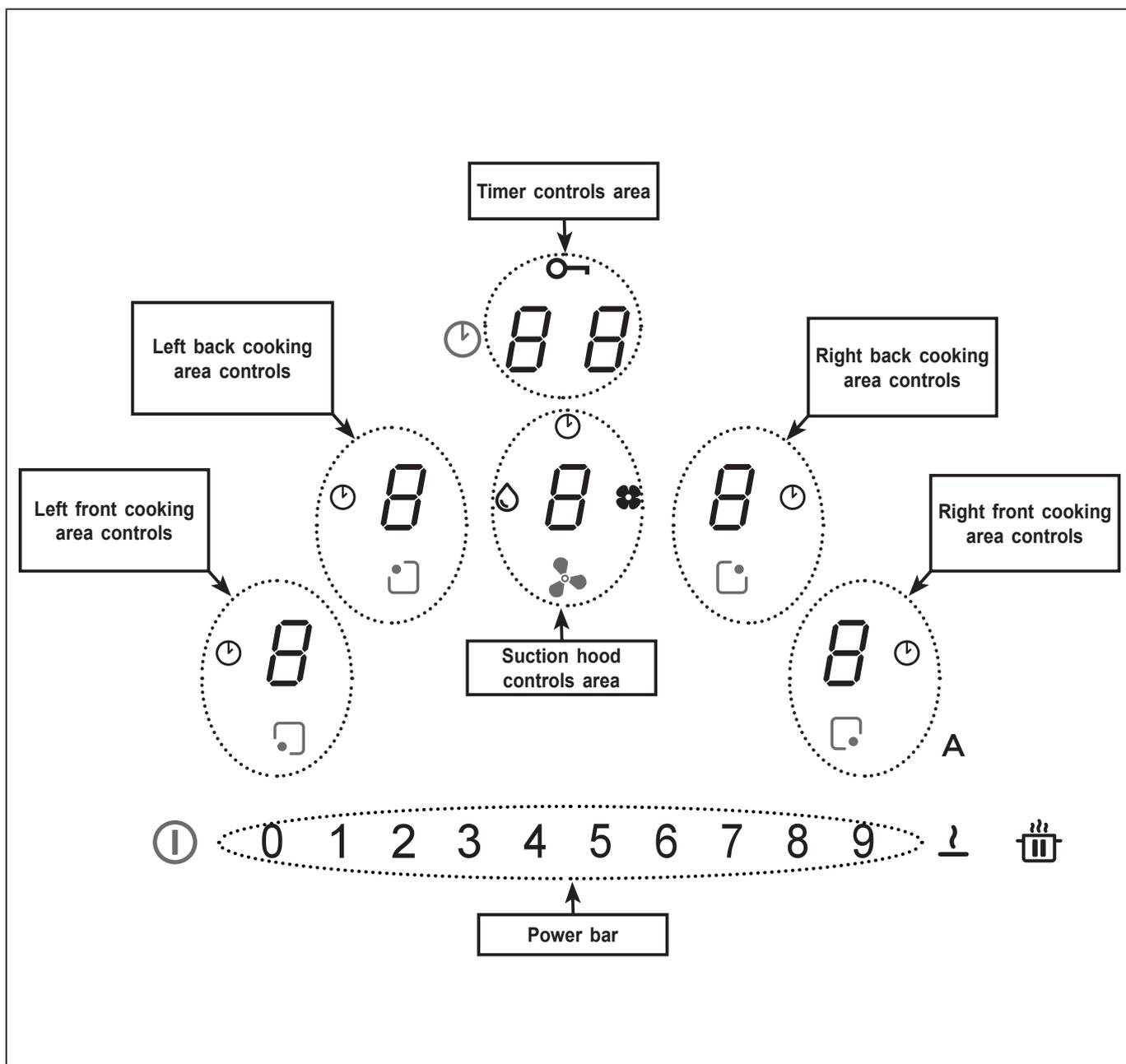
The controls for the cooking areas, suction hood and timer can be activated by pressing on the reference Digit 8. The Digit lights up more intensely to confirm the operation.
