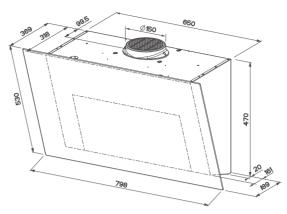
To be installed at a minimum distance from the hob of 45 cm.
